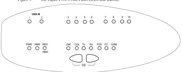
Figure 4 The Cajun P118 Front Panel LEDs and Buttons
